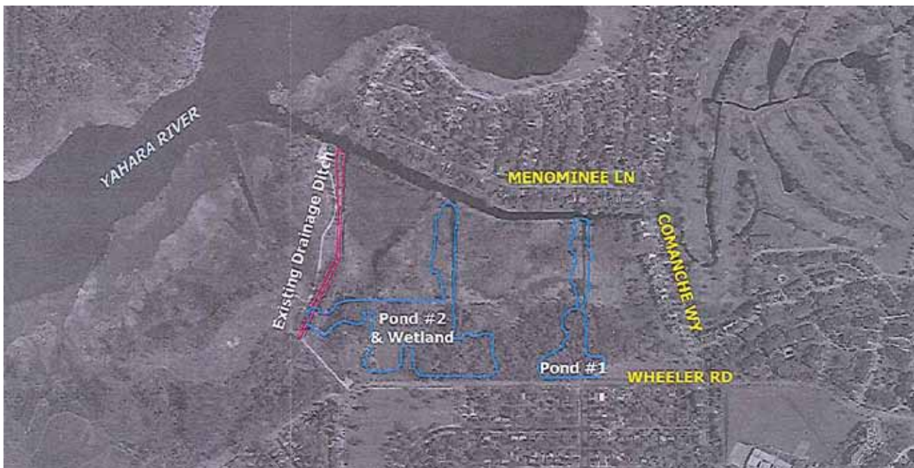
The proposed retention ponds and restored wetland will keep sediments and other pollutants from reaching the Yahara River at Cherokee Marsh. (City of Madison Engineering Division drawing.)
